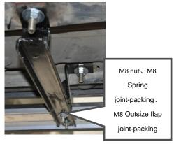
D. Adjust the boards to be perfect fitment. Install back the skid plate which be taken off before installation.
