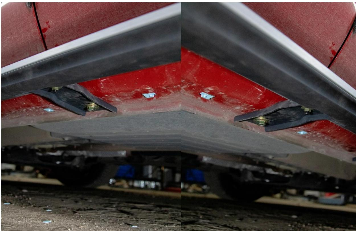
**\*If the side step doesn't fit well, cut the edges of the running board (the side from the back of the car)**
