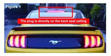
2. Use Accessory 1: upper brake light adapter cable for USDM
