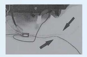
Pull out the bulb and change the new one (bulb type: 16.5v/0.27W)
