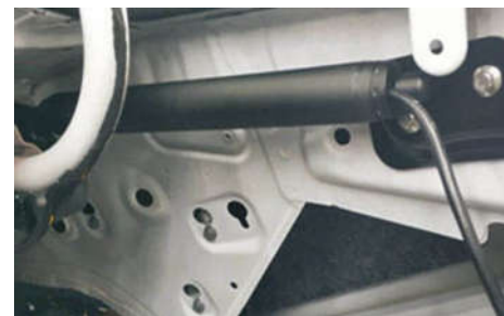
11. Install our electric pole ("L" on the left and "R" on the right)
