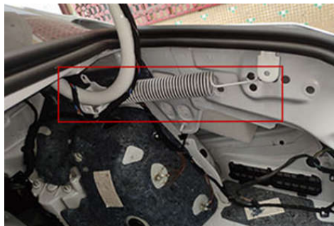
3. Remove the original car body spring (same left and right)
