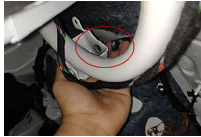
7. Remove the hanging spring plastic parts (same for left and right)
