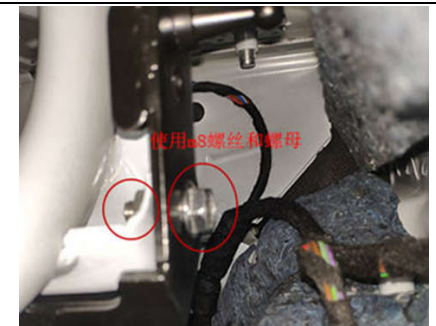
10. Use our M8 screws and nuts to lock in the original hanging spring position (same left and right)
