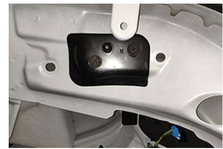
6. Install our body bracket (left of "L" and right of "R")
