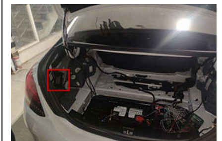
24. Connect the corresponding wire harness to the control box, and fix the control box
