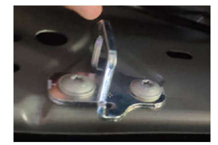
12. Remove the original car lock hook
