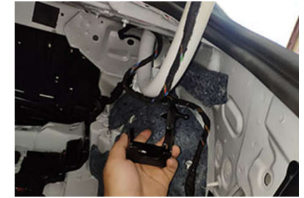
8. Set our swing arm bracket to the original spring position (same left and right)
