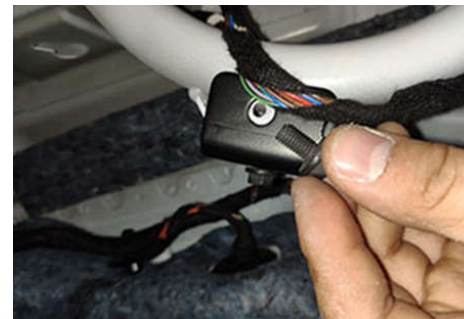
9. Use our M6 screws to tighten (same left and right)
