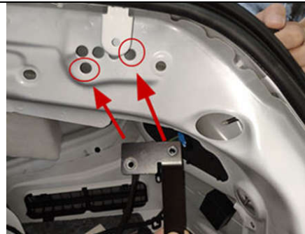
4. Put our nut washer into the marked hole in the picture (same left and right)
