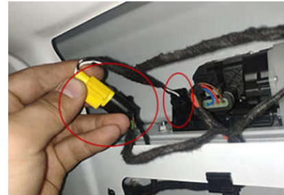
18. Unplug the original car lock plug and connect it to our wiring harness
