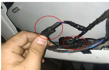
17. Unplug the original car lock plug and connect it with our line
