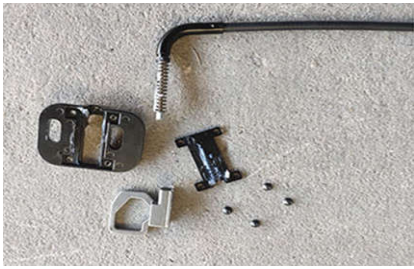
13. Disassemble the lock plate of our electric suction zipper
