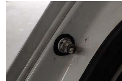
9. Add a gasket of our company on the basis of the ball head of the original car (same left and right)
