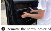
1 Remove the screw cover of the interior trim panel
