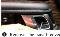
3 Remove the small cover plate of the inner handle and remove the screw
