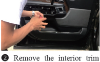
2 Remove the interior trim panel screws
