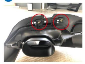
Then use self-tapping screws to attach the tailpipe bracket and tail lip.
