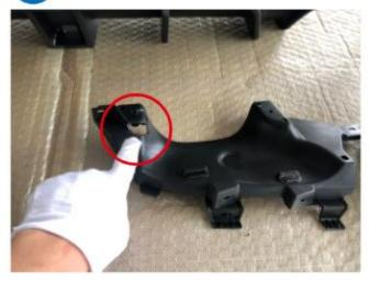
Refer to the example picture, use professional tools to cut off part of the installation bracket at the position shown in the picture in order to match the tail pipe.
