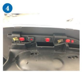
Install the reflector, slightly secure it in the correct position on the inside of the bracket, and then connect the tail lip to the rear bumper.
