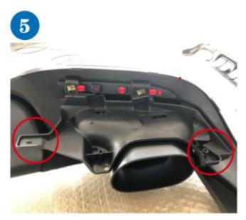
After you have mounted the tail pipe with the bracket on the diffuser, mount the diffuser on the rear bumper.
