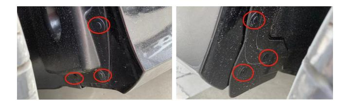
**Step 3:** Remove the plastic nuts from the underside of the original car and keep them for later re-installation (as shown on photos below).
