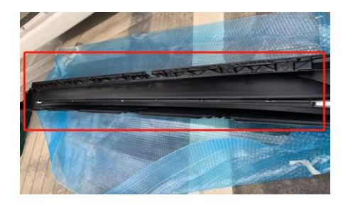
**Step 6:** Take out the No. (2) bracket from the package and install it in the corresponding side holes, then secure it with No. (5) screws (while tightening, push the side skirt upward to facilitate the installation of the side
