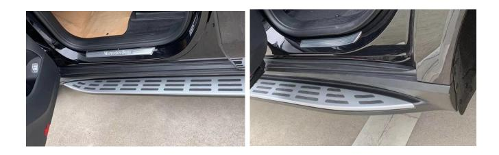
**Step 9:** Cover the secured side step with the No. ③ plastic small cover plate to complete the installation. (as shown on photos below)
