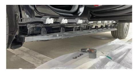
**Step 7:** Remove the white plastic clip at the front of the original side skirt and install it in the corresponding position on our No. (1) side step. (as shown on photos below)
