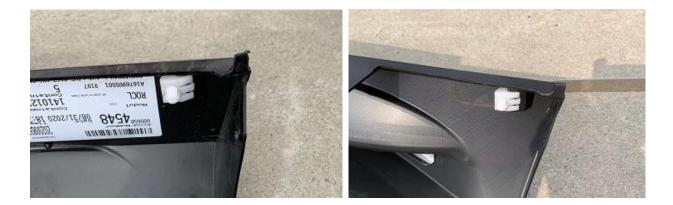
**Step 8:** Install the No. (1) side step onto the vehicle body. After aligning the holes, first secure the lower clips by tapping them into place, then fix the upper part. Finally, re-install the plastic clips removed from the front and rear. (as shown on photos below)
