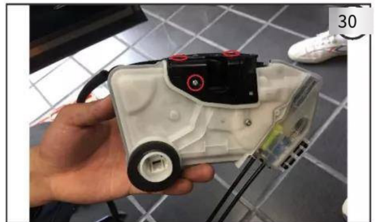
8. Fix the electric suction lock core with the 3 fixing screws of the original lock core (as shown in the red circle in Figure 30)
