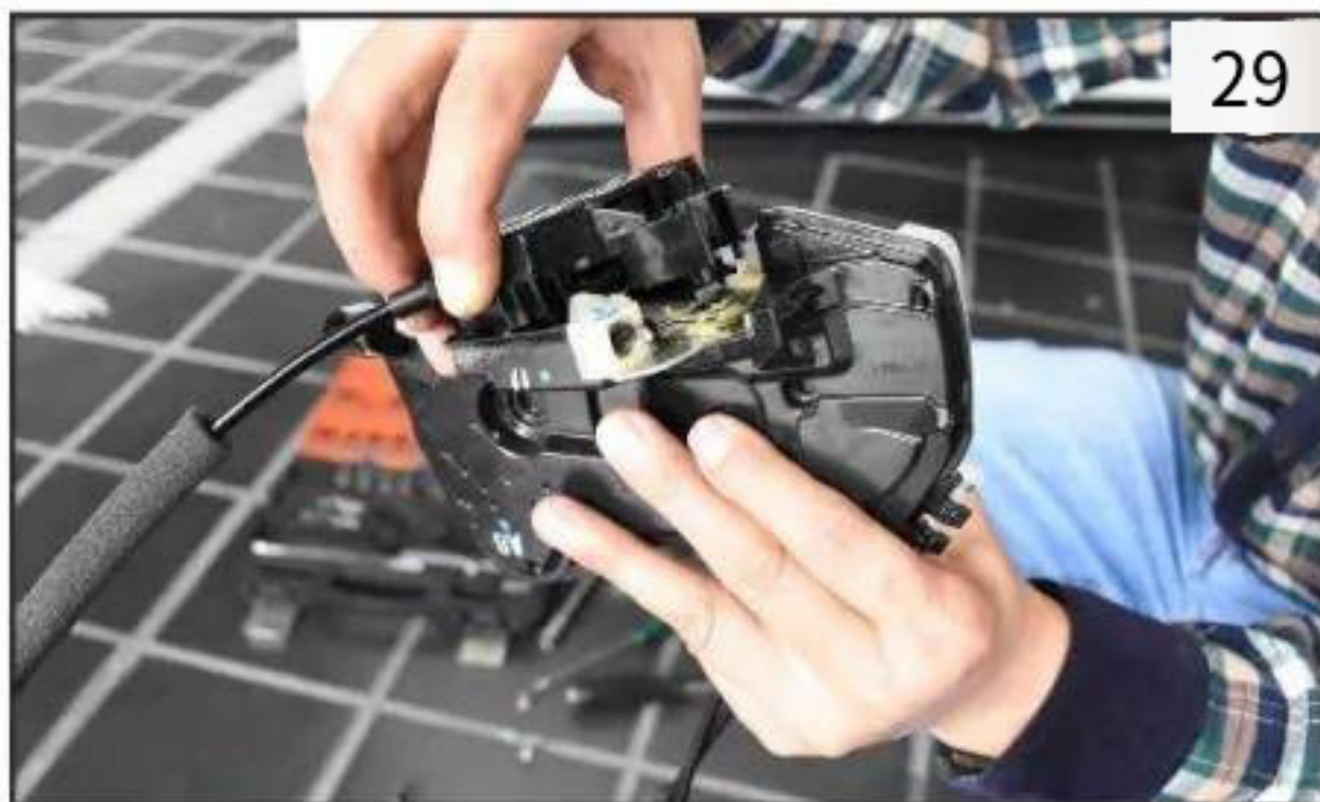
7. Install the electric suction door lock core on the original car door lock (Figure 29)
