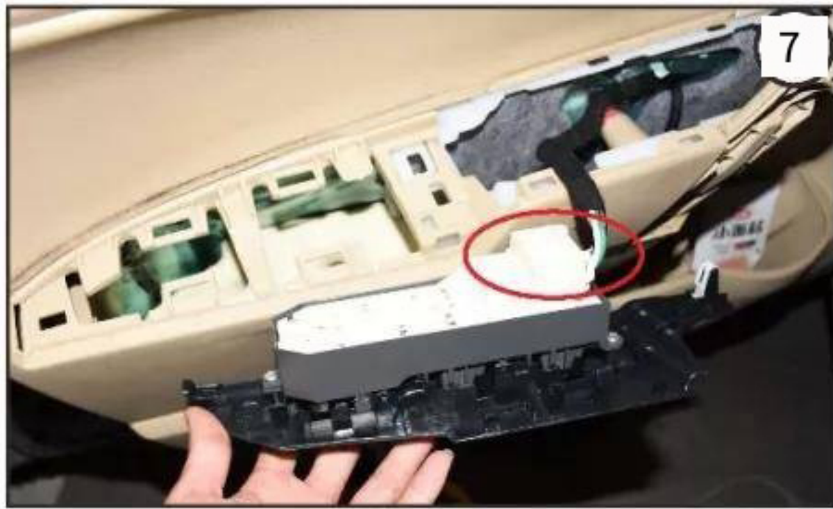
7. Remove the connecting signal on the back of the glass lifter cover plate (as shown in the red circle in Figure 7)
