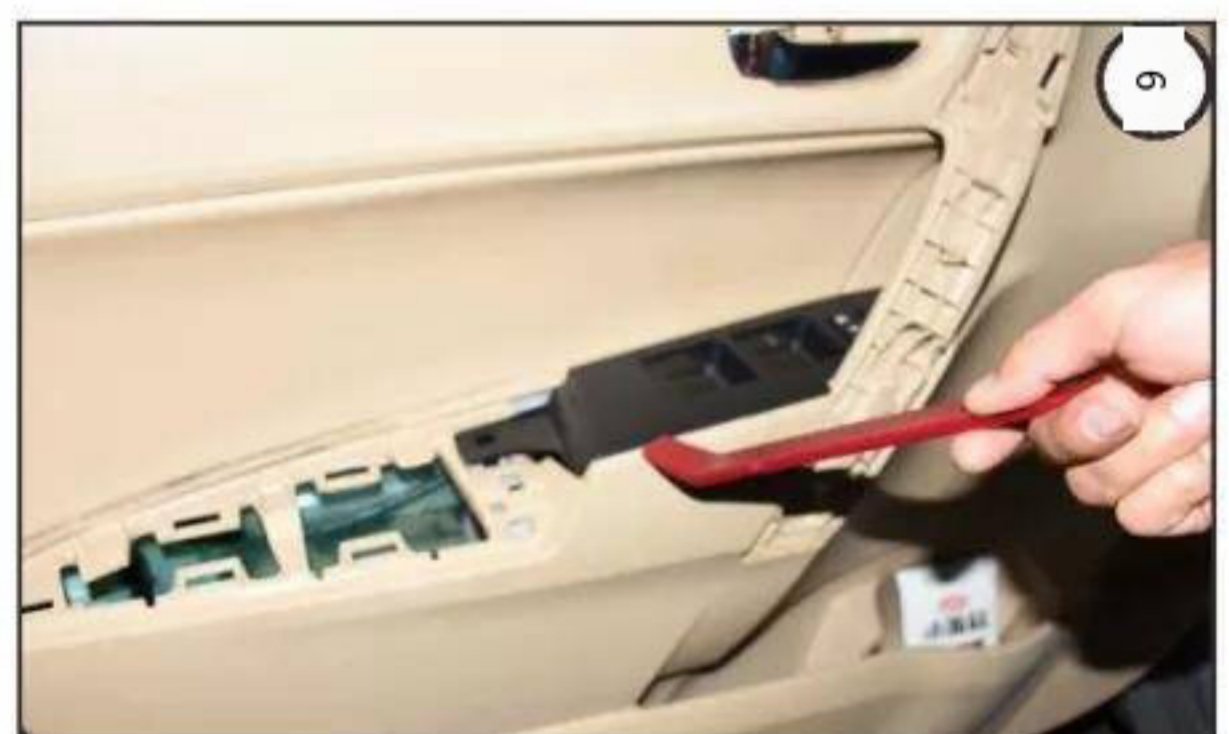
6. Carefully pry open the glass lifter cover with a pry knife (Figure 6)
