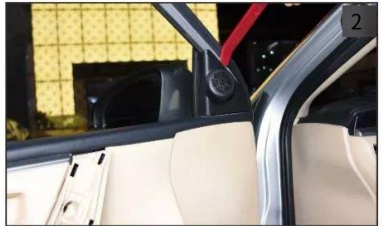
2. Use a pry knife to carefully pry open the horn decorative plate (Figure 2)
