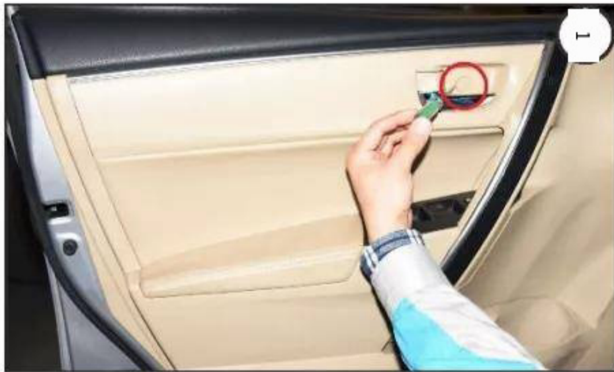
1. Use a pry knife to carefully pry open the inner door handle decorative plate (Figure 1)
