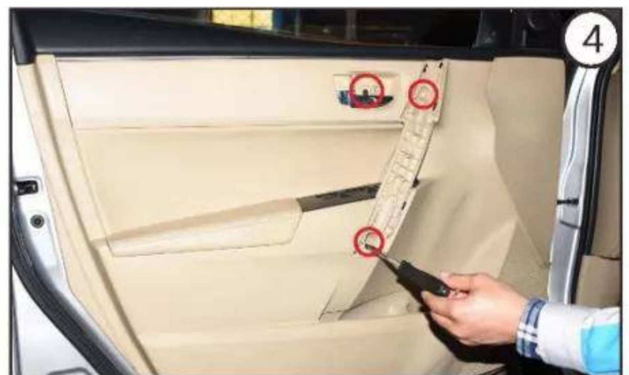
4. Use a screwdriver to remove the three fixing screws shown in the red circle in Figure 4.
