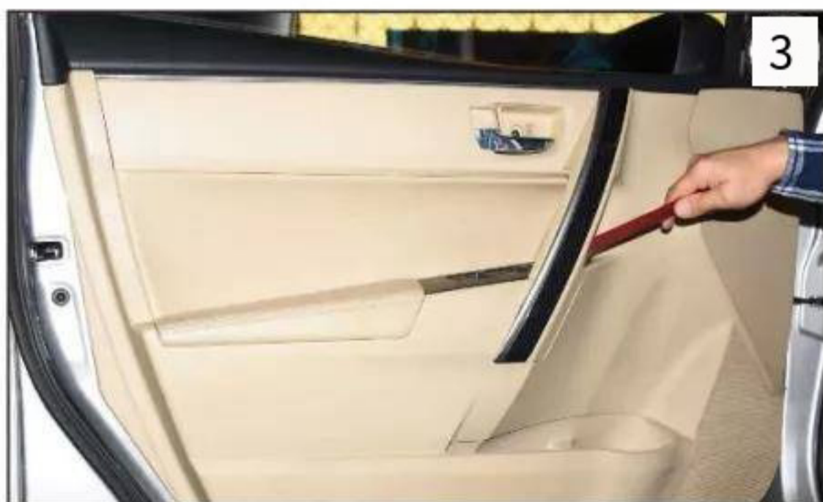
3. Carefully pry open the decorative bar of the handrail with a pry knife (Figure 3)
