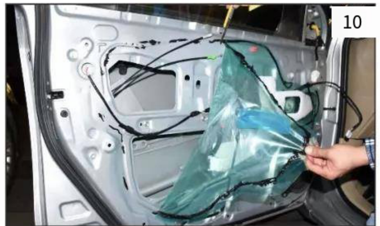
10. Use a utility knife to carefully mark the soft glue along the edge of the soundproof cotton (Figure 10).
