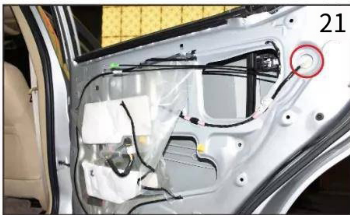
9 Remove the connector plug (shown in the red circle in Figure 11).
