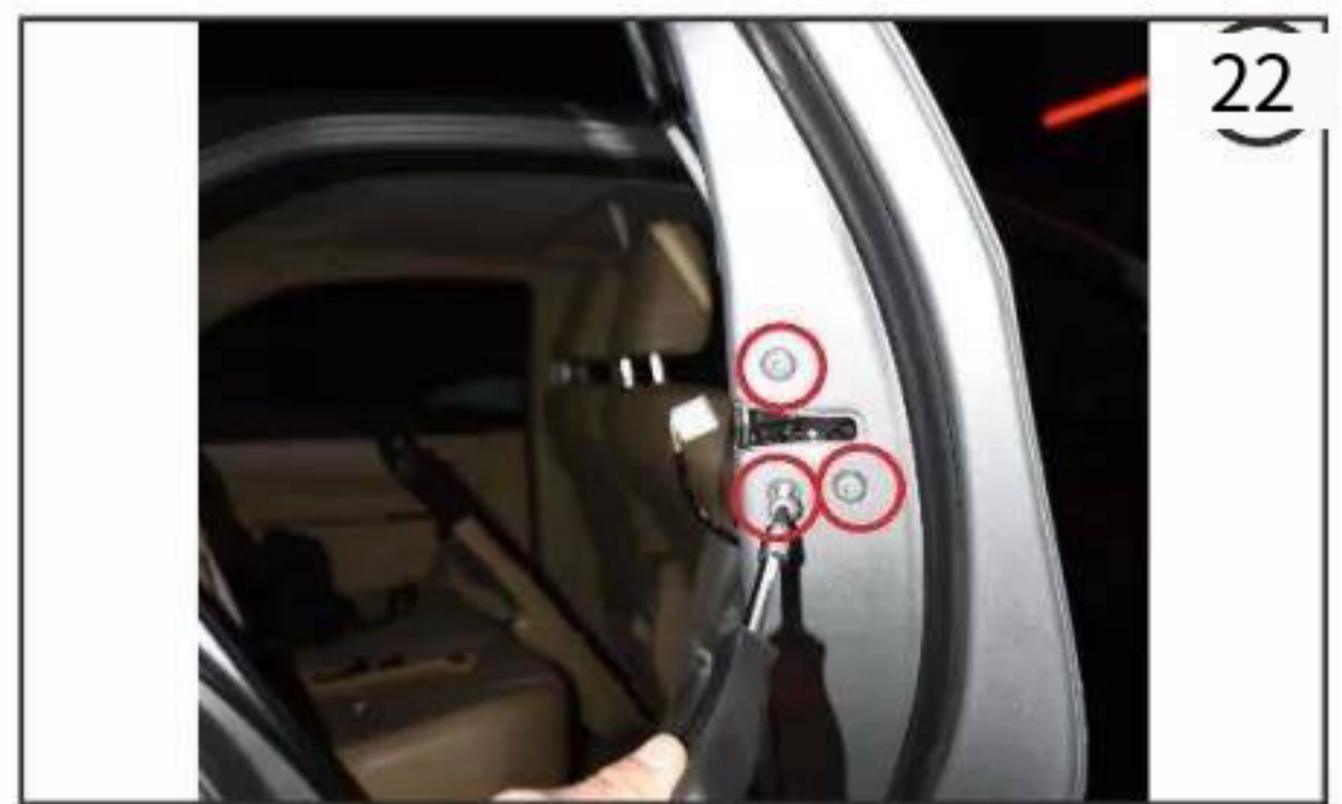
10. Remove the three fixing screws as shown in the red circle in Figure 22, and then remove the original lock head.
