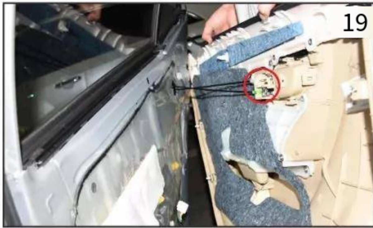
7. Remove the two cables on the back of the door trim plate (as shown by the red circle in Figure 19)
