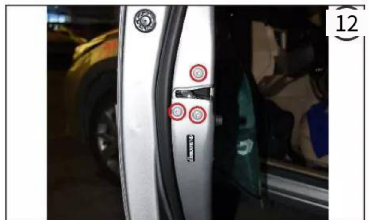
12. Remove the three fixing screws as shown in the red circle in Figure 12, and then remove the original lock head.
