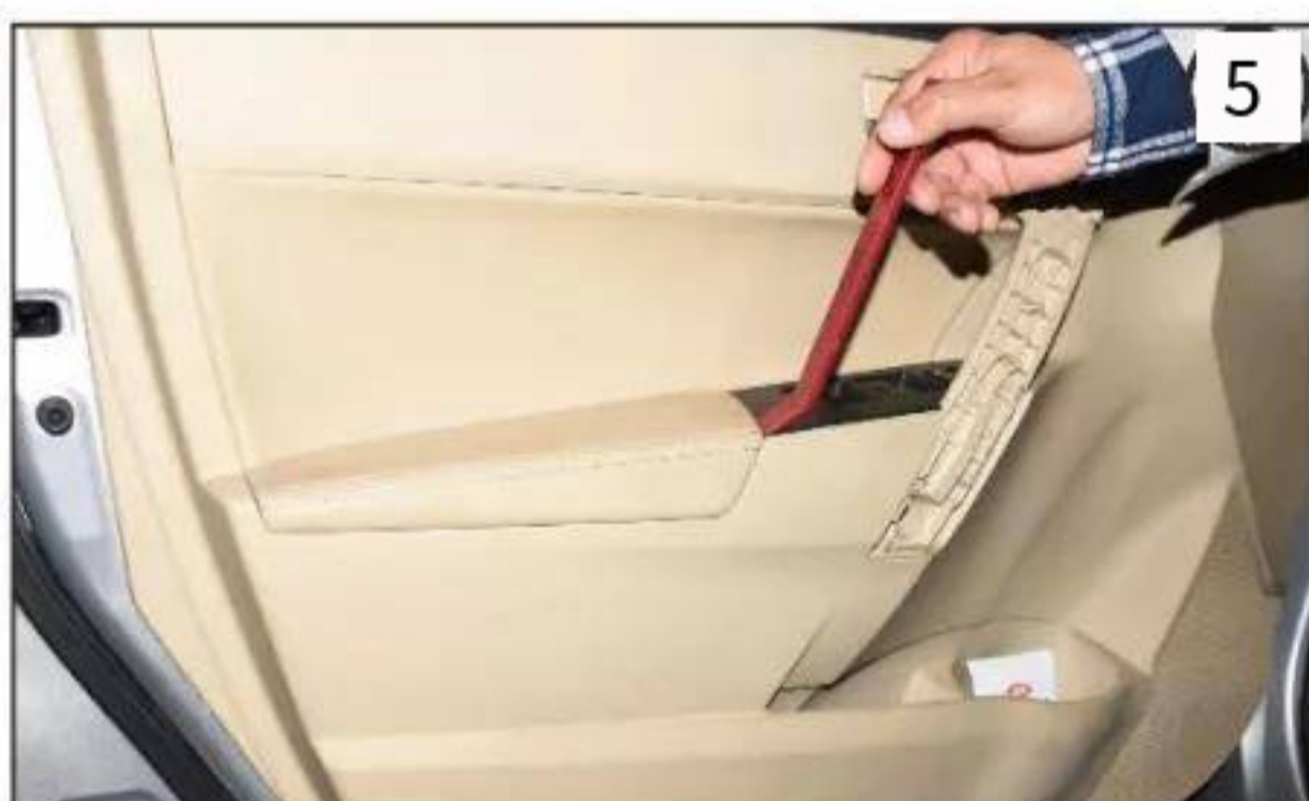
5. Use a pry knife to carefully pry open the armrest decorative board (Figure 5)
