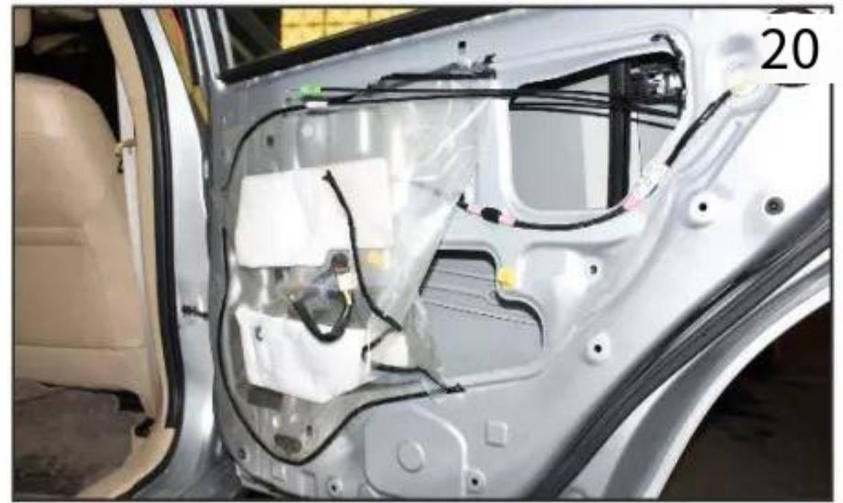
8. Use a utility knife to carefully mark the soft adhesive along the edge of the soundproof cotton (Figure 20).
