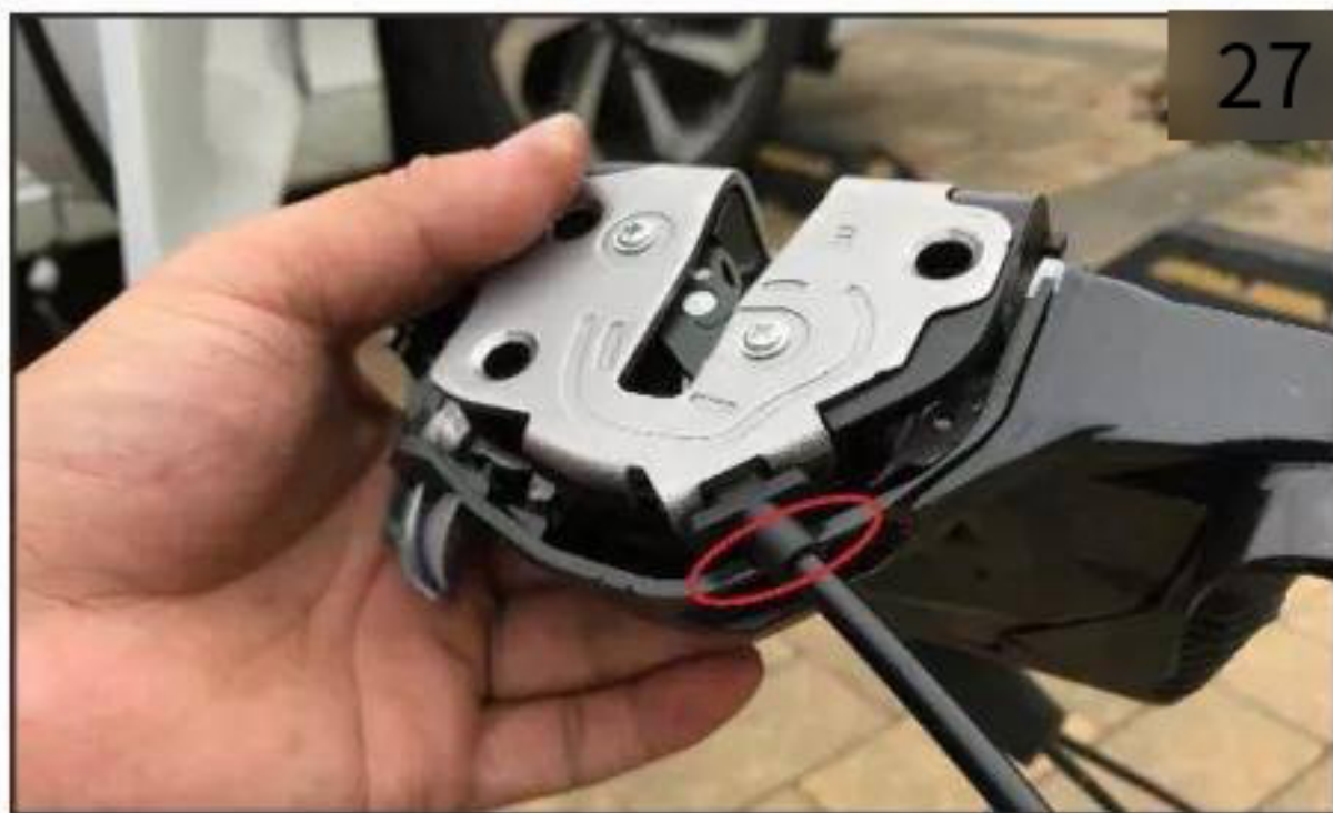
5. Take out the core assembly of the electric suction door lock, put part of the lock core on the car door lock (Figure 27), and record the approximate position of the cable of the electric suction door lock core (as shown in the red circle in Figure 27).
