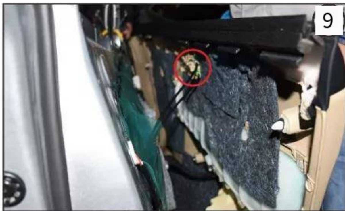
9. Remove the two cables on the back of the door trim plate (as shown by the red circle in Figure 9)
