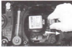
1 Disconnect the power plug
